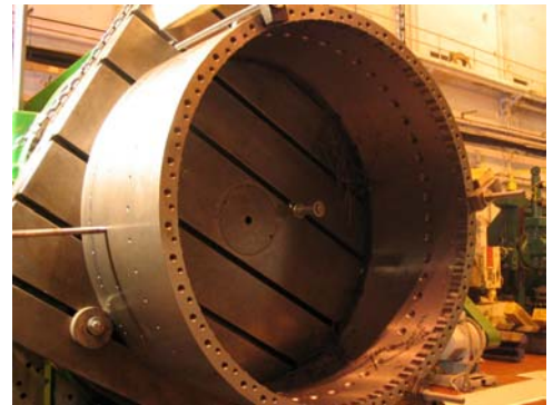
New Diode Wheel after Machining
