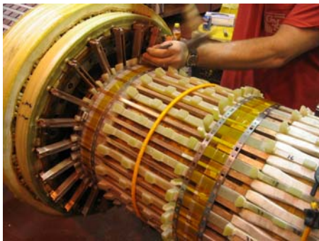
Phase Lead Modification
