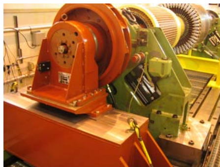
PMG Output Testing @ 3600 RPM
