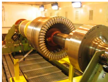
Exciter Loaded in High Speed Spin Pit
